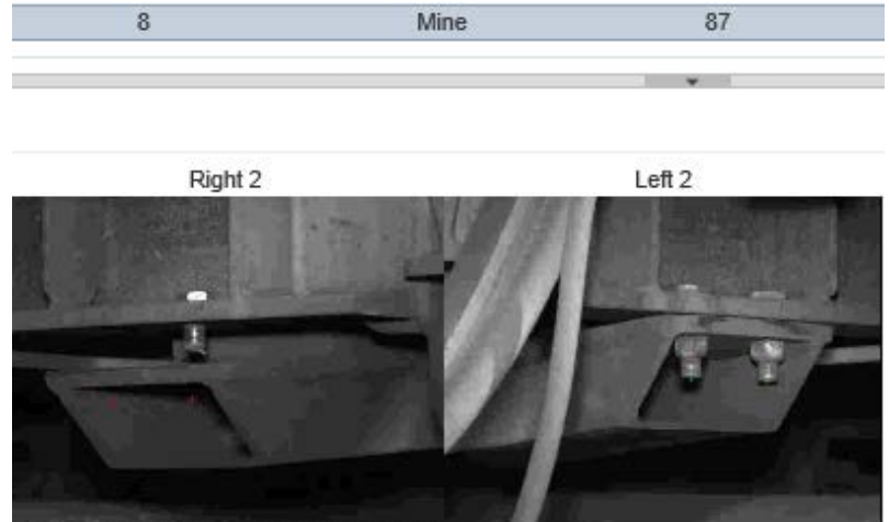
Figure 1. Photograph of retainer bolts from iron ore car
