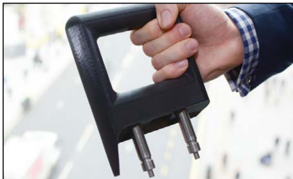
3D Printed Grab Handle Produced by Angel Trains, DB ESG, and Stratasys (Source: GlobalRailwayReview.com)
