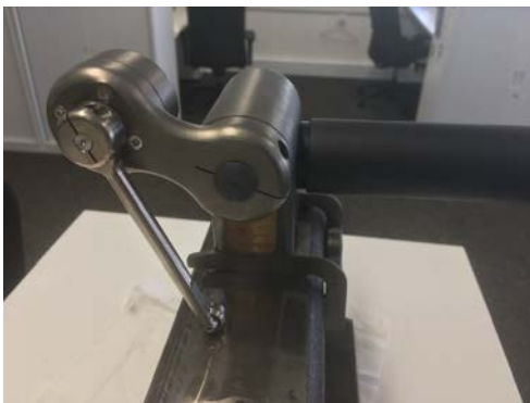
Figure 2. Mini-Prof by Greenwood Engineering Measuring the Rail Head Profile
