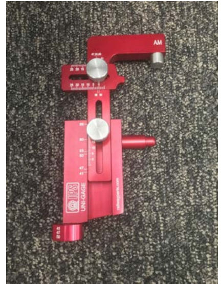
Figure 1 - Uni-Gauge which measures vertical and side wear at specified locations of the rail head
