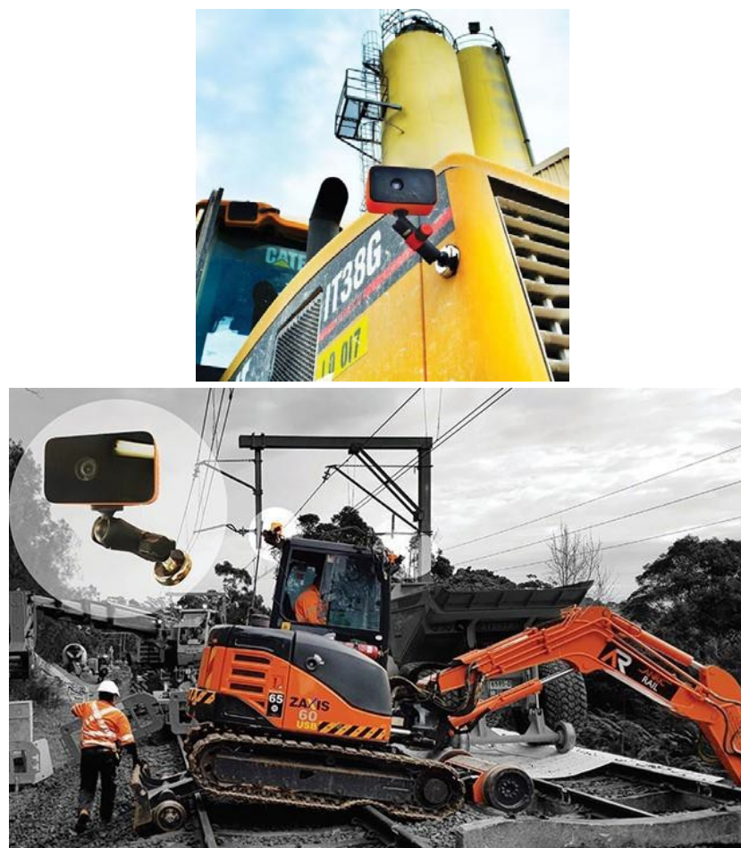
Figure 1: Toolbox spotter positioned on pieces of plant to alert the driver of humans or foreign objects in proximity (Photo: Laing O'Rourke)
