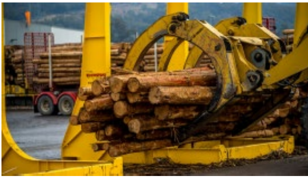
Figure 4: Loading a Bookend in Brighton Intermodal Yard
