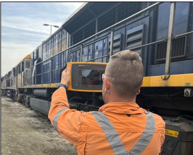
The interface allows technicians to isolate the sound frequency of the leak, to filter out loud background noise.
