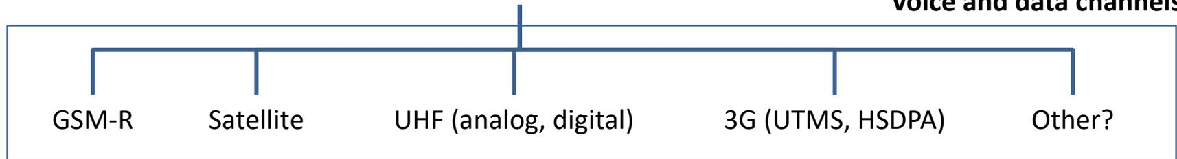
ICE provides a single system on a locomotive that can communicate through multiple channel options, depending on the solution appropriate to the operations. ICE was initially equipped with systems relevant at the time of fitment, however is able to be upgraded and expanded to accommodate future radio systems as they are deployed.
