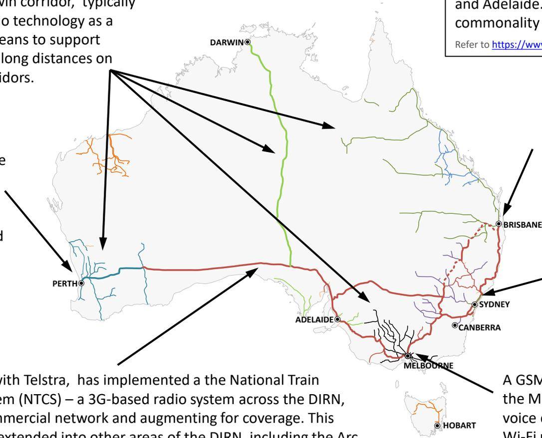
TMR/QR is implementing GSM-R on the SEQ rail network, as part of the cross River Rail / ETCS Inner city initiative. This will support ETCS L2 operations as well as provide voice communications.
