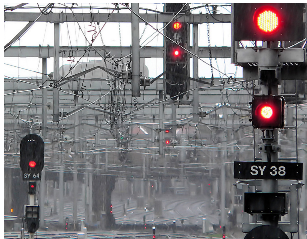
This image illustrates how a driver may read across to a non-target signal.
