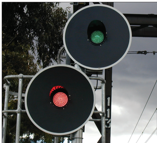
3 position automatic signal. In Victoria the above signal shows proceed at normal speed but in NSW this is a cautionary signal
