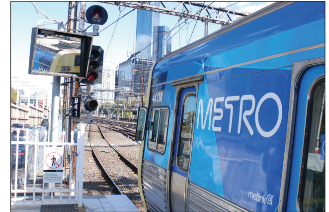
A mirror used for driver only operation - RTO's need to consider specific risks in relation to SPAD management
