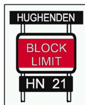
Example block board used in NSW - the design and sighting of limit boards like signals should be carefully considered. This is an example of a well designed block board.
