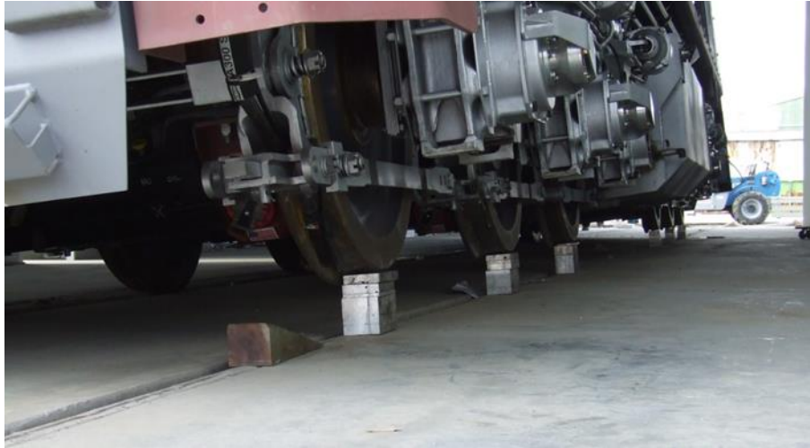
Figure C 1 - Static kinematic test setup (wheels packed to maximum test cant)
