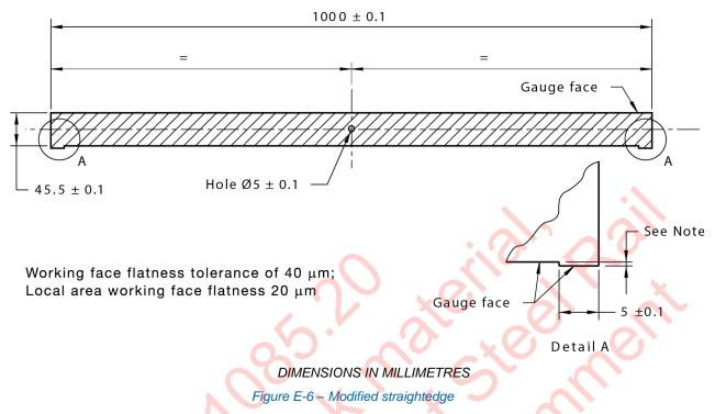
A separate modified straightedge shall be used for each surface alignment tolerance grade (see tables 2.1, 3.1 and 4.1). The size of the lug (detail A) is 0.3 mm, 0.5 mm, or as defined by the purchaser, and shall be stamped on the straightedge. Tolerances for the lug shall be  $\pm 0.05$  mm.
