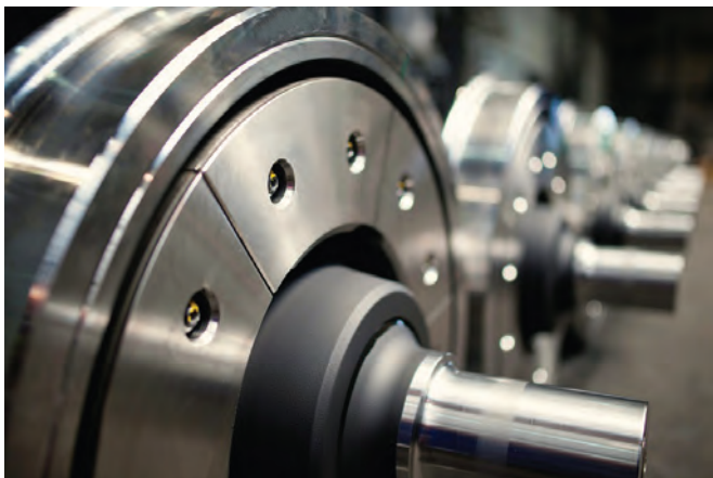
Figure 25 Wheels with dampers installed (70)
