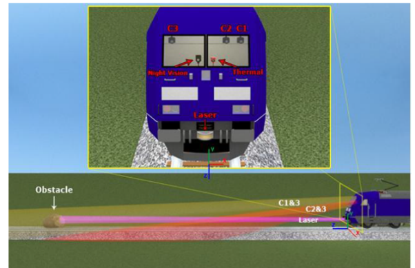
Figure 3: Concept of SMART multi-sensor obstacle detection system. (Top) Front view of sensors mounted on locomotive, (Bottom) Side view of range sensors and obstacle detection scene
