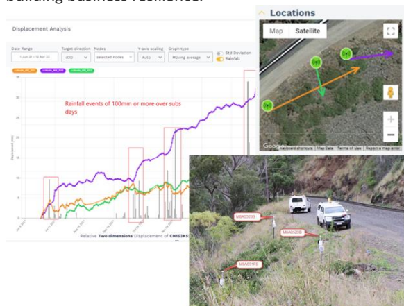
Figure 2 –Displacement analysis graph (left) showing real-time data recording from embankment monitors (right) after subsequent days of rainfall.
