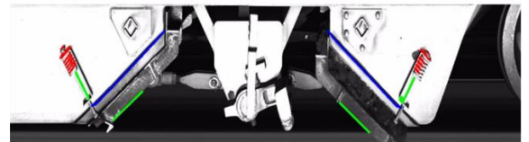
Figure 2: A failed hinge causing a coal wagon door to open in traffic automatically detected by the MVA
