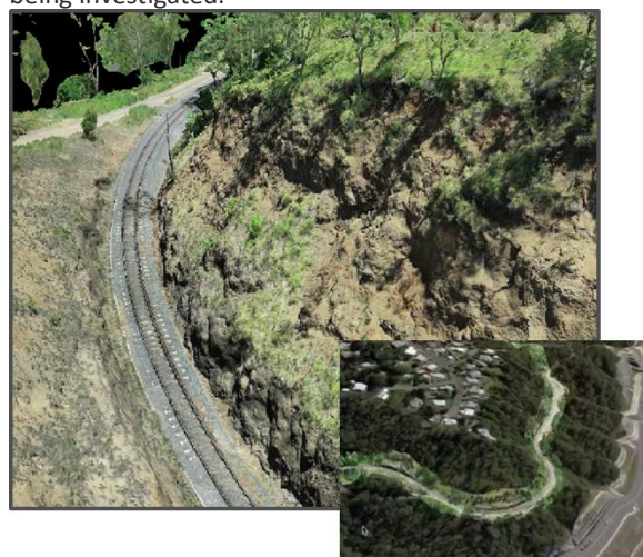
Figure 1 – A graphic from Queensland Rail's digital twin model established using Photogrammetry and LiDAR
