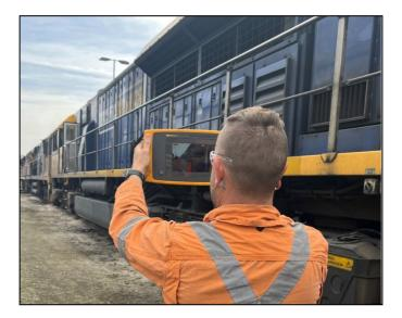
The interface allows technicians to isolate the sound frequency of the leak, to filter out loud background noise.
