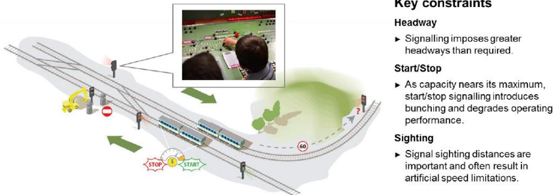
Figure 1 ETCS Level 1 with Conventional Signalling
