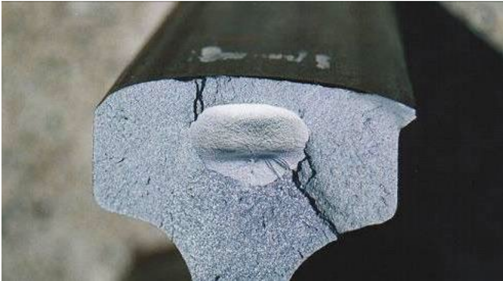
Appendix Figure D.7 Transverse defect
