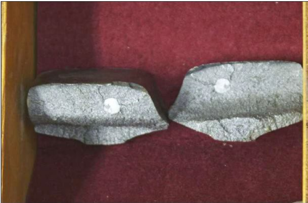
Appendix Figure D.6 Shatter crack
