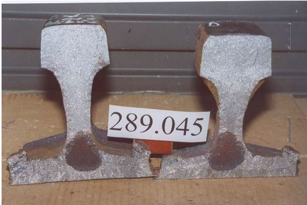
Appendix Figure D.11 Weld defect
