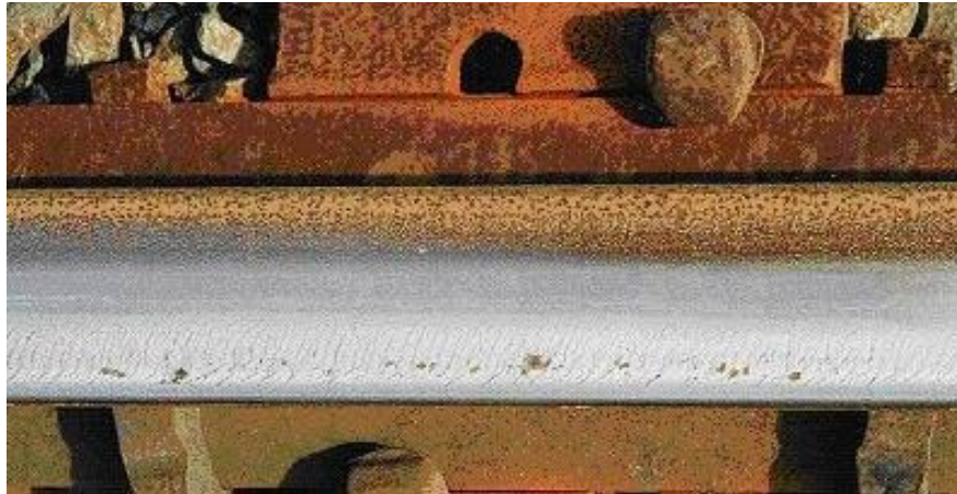
Appendix Figure D.18 Gauge corner cracking
