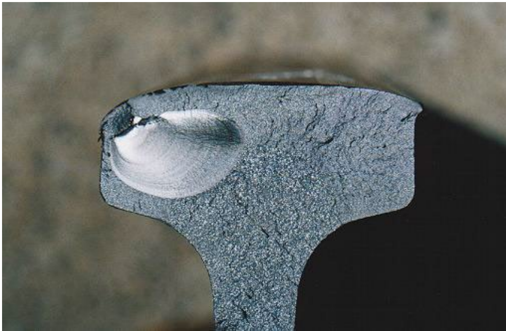
Appendix Figure D.8 Transverse defect from shelling
