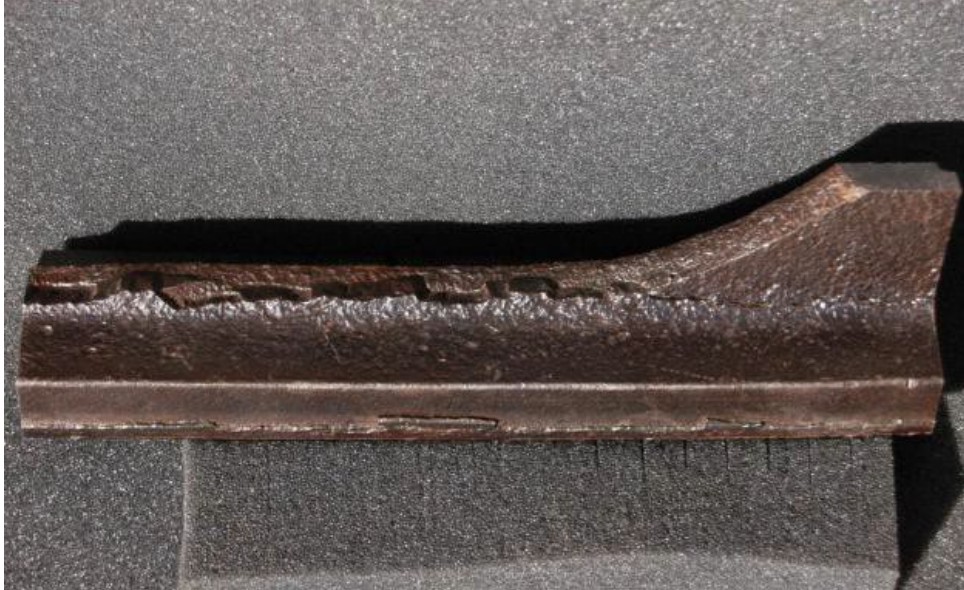
Appendix Figure D.20 Head web separation
