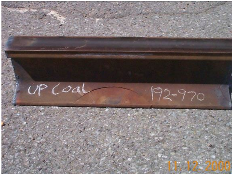
Appendix Figure D.12 Broken foot
