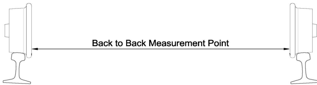
Figure 4 Measurement point for wheel back to back
