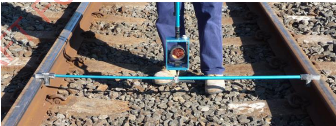
Appendix Figure C-5 Track bar used to measure track centreline
