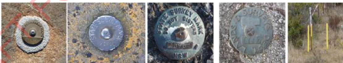
Appendix Figure D-4 Other types of permanent survey control marks
