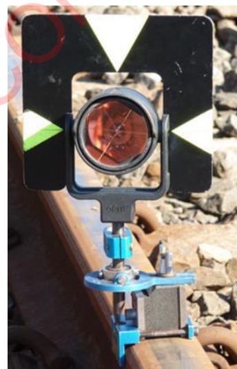
Appendix Figure C-4 Magnetic rail prism
