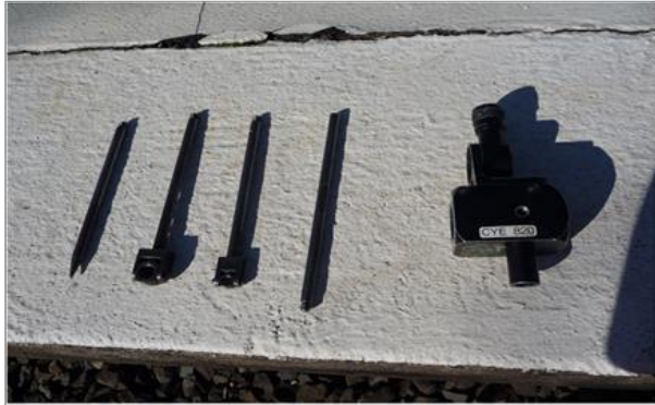
Appendix Figure C-1 Offset prism and associated attachment arms
